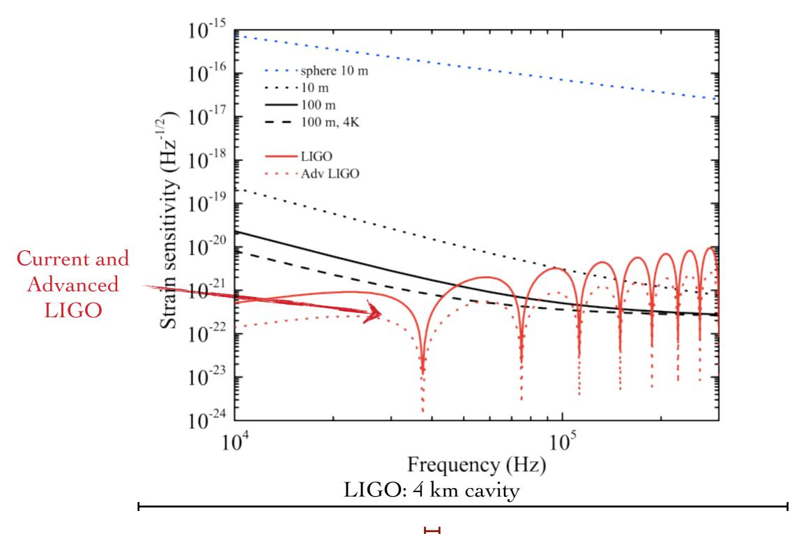
Current setup: 100 m cavity
