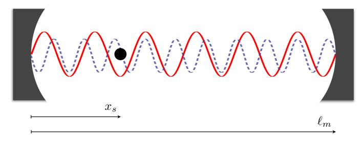
Gravitational wave changes the physical distance between masses  $L = L_0 \; (1 + h \; cos\omega t)$
