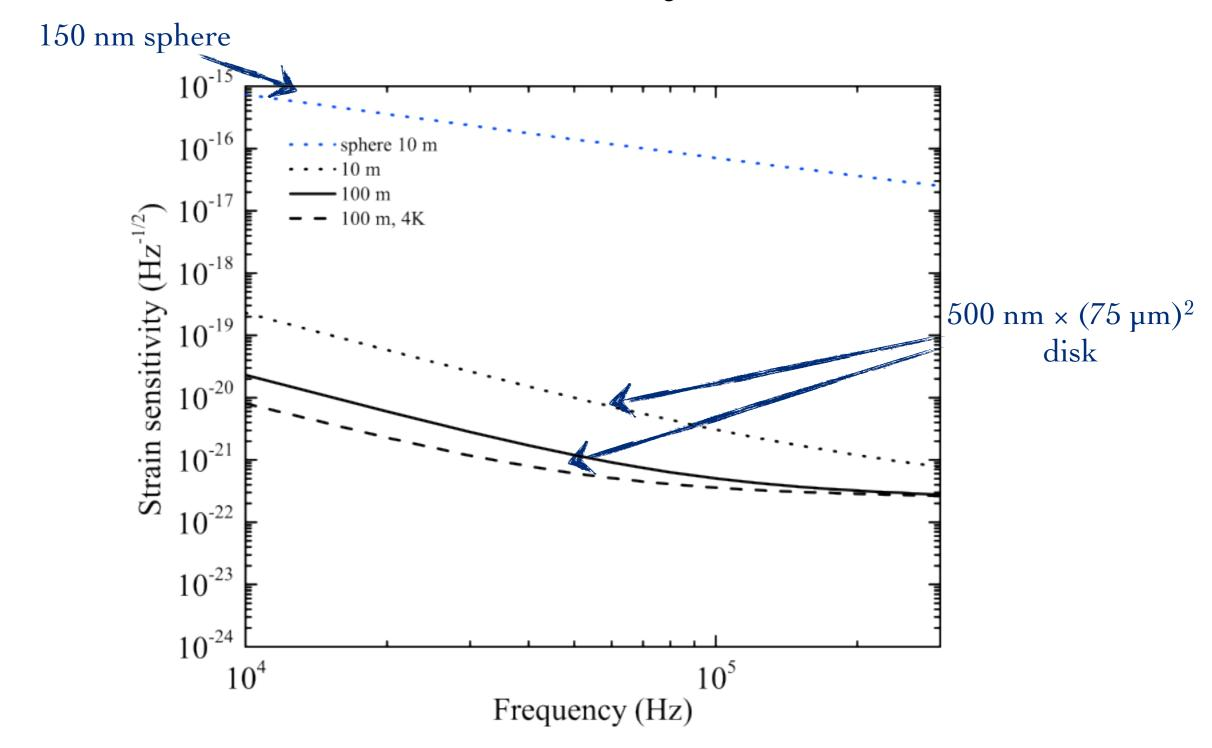
Radical change in sensitivity between the two geometries due to difference in mass and in light scattering properties
