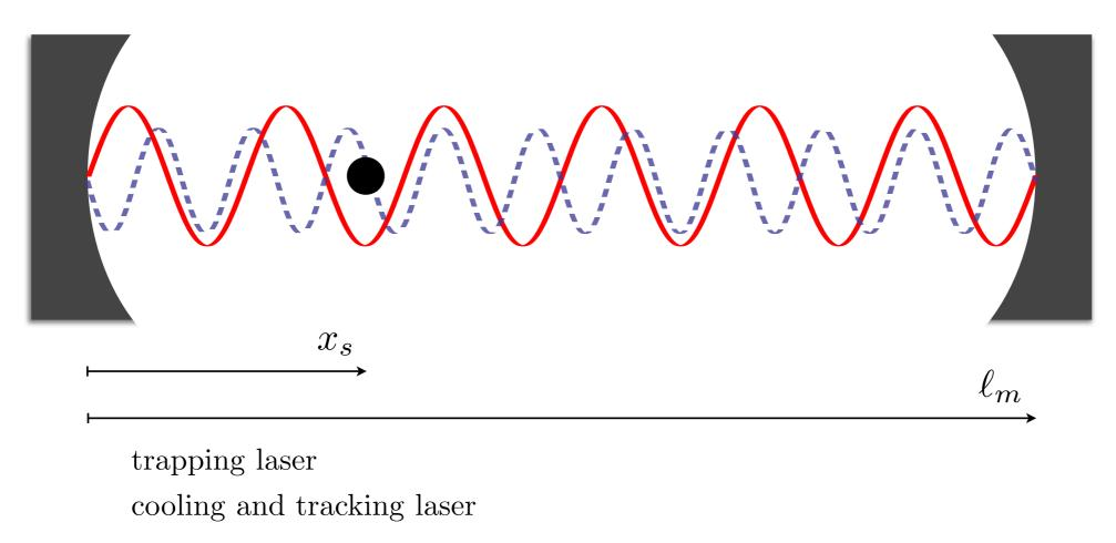
• Fused silica sphere (r = 150 nm) or disk (d=500 nm, r=75 µm) sensor in optical cavity of 10-100 m in size
