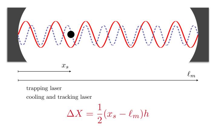
• Laser intensity changes resonant frequency of the sensor: Tunable resonant GW detector
